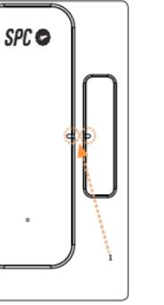
**EN** · Once the sensor is added to the application, install it in the place you want. To do this, peel off the double-sided strips and place both parts on flat, clean surfaces. Keep in mind that both notches must coincide (1) and that there cannot be a distance greater than 15mm between both parts of the sensor when the sensor is closed.
