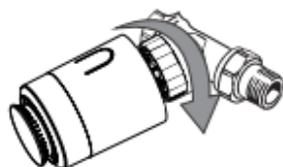
Briefly press the valve control dial. The display will begin to flash "LA" again while it self-adjusts.
