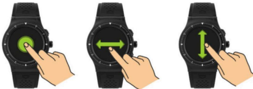
With the movements mentioned you can browse between the horizontal and vertical menus. From the main screen you can browse into the inferior and upper menus using the wheel on the side of the watch. To confirm your choice, press this same button.
