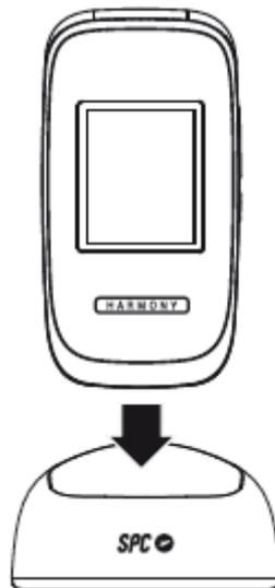
To charge the handset, connect the power supply to the charging cradle and to any power socket in your home. Check the orientation of the connector and do not force the connection if it is not immediate. Place the phone on the charging cradle.
