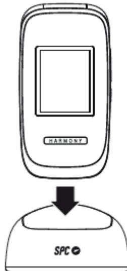
To charge the terminal, connect the power supply to the charger base and to any socket in your home. Check the orientation of the connector and do not force the connection if it is not immediate. Place the phone on the charging cradle.
